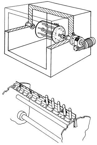
FIG. 2 Uniaxially Rotated Specimen Holder—Drum Rotator
