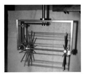
FIG. 1 Biaxial Ferris-Wheel-Type Rotator
